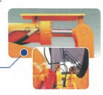
Auto boom kickout device stops the boom at preset height automatically to protect the operator from mechanical impact for reduced operator fatigue
